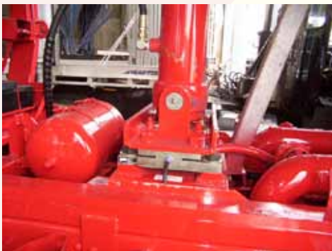
RAM LOADCELL INSTALLATION
