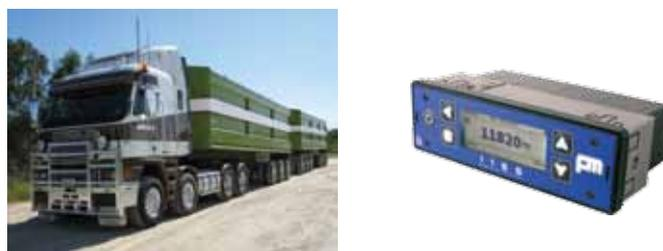
**BulkWeigh** is a highly accurate loadcell system specifically designed for conventional tipping vehicles. The loadcells are mounted under the hydraulic lift ram and the rear hinge bar. This system is suitable for rigid, semi-trailers and rigid drawbar vehicles. Features: AxleWatch for monitoring load spread, and TipWatch to prevent unsafe tipping on uneven ground.
