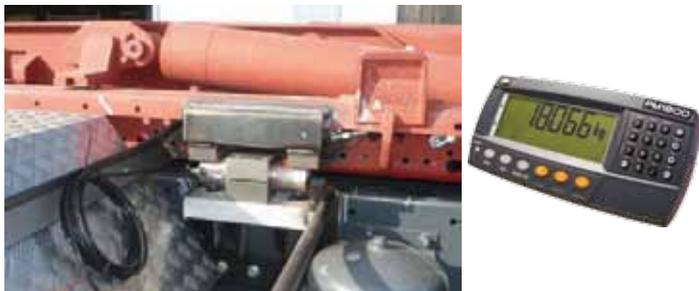
The LFT1500 approved body weighing system is a high-accuracy, legal-for-trade system for invoicing at the point of collection. LFT1500 comprises four or six approved loadcells which are mounted between the chassis and body, an inclinometer and the in-cab indicator, now trade approved in Australia to class IIII (NMI No. 6/9C/301).
