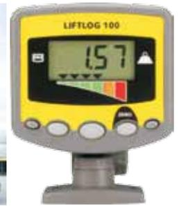
The **ForkWeigh** forklift weighing system is designed for use on a variety of forklift trucks in dispatch yard or warehouse applications. Using an electronic sensor to measure hydraulic pressure on the lift cylinder the **Liftlog 100** displays live weight in tonnes or kilograms. In the event of an overload an internal or (optional) external warning alarm warns the operator.
