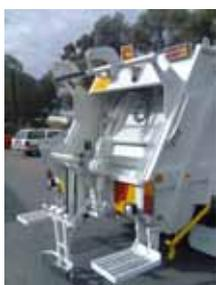
**BinWeigh** is a wheelie bin weighing system installed onboard a waste collection vehicle and gives waste managers much more meaningful source data to manage their collection routes. It gives unprecedented productivity gains and improved waste information right across the waste operation.
