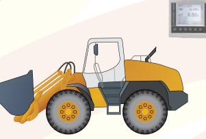
Loadmaster 8000iX: dual-sensor nonapproved system with target weight entry. last bucket tip-off, data management and a printer option.
